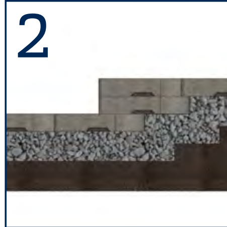
Install Base Course
