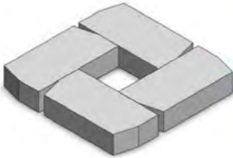
Place the grid on a prepared surface
